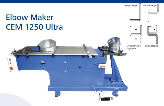
The Elbow maker CEM 1250 Ultra was developed for the production of segmental elbows and similar articles in segments (reductions, caps, ect.). Crimping the segments and closing the flange creates a airtight seam, which meets every needs. Due to their flexibility and the simultaneous use of flanging and closing station this machine is ideal for mass production and custom manufacturing.
